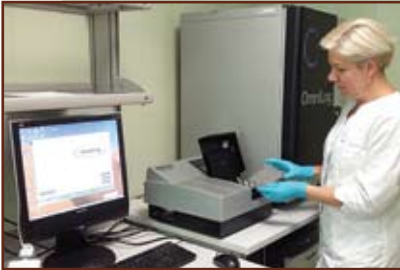
Community-level physiological profiling of soil microorganisms using a Biolog system
