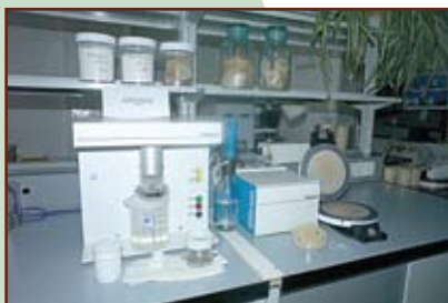
Determination of grain quality – gluten content and gluten index (GI) (GLUTOMATIC system, Perten)
