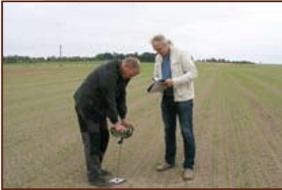
Determination of depth and thickness of soil plough pan
