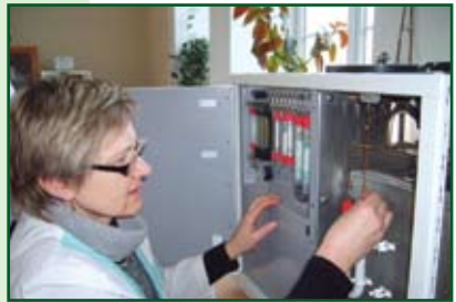
Plant and soil analyses – determination of C, N, S by the Dumas method (Vario EL III, Elementar)
