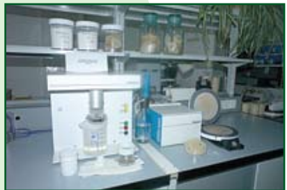
Determination of grain quality – gluten content and gluten index (GLUTOMATIC system, Perten)
